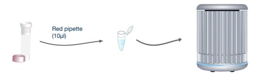
Take great care when setting up your positive control. The positive control template has the potential to give you a false positive signal in your other samples. Set positive controls up last after all other sample tubes are closed. Always change pipette tips between samples. You may even choose to set up positive controls in a separate room.
