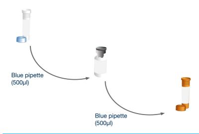
Use the blue pipette to transfer 500µl\* of the oasig Master Mix resuspension buffer into the tube of lyophilised oasig Master Mix and mix well by gently swirling. Then transfer all of that master mix into the brown tube labelled C.trachomatis primers/probe.
