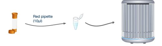
For every reaction to be run, use the red pipette to add 10µl of your Ehrlichia\_spp reaction mix to every tube.
